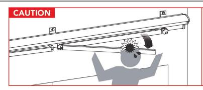
The awning arms contain tensioned cables. Always use caution, securely tie the awnings arms to the awning when performing installation, adjustments, or repairs. Sudden movement of tension arms can result in serious personal injury, product and/or property damage.
