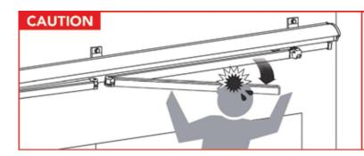
The awning arms contain tensioned cables. Always use caution, securely tie the awnings arms to the awning when performing installation, adjustments, or repairs. Sudden movement of tension arms can result in serious personal injury, product and/or property damage.
