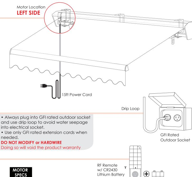
**SPECS** Class Volts 120 205 Watts 1.92 **Amps** 40Nm 13r/min 3.75kg Other
